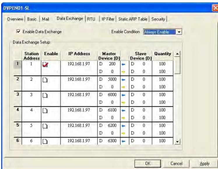
3. Choose 'Enable Data Exchange,' select the execution mode as 'Always Enable.' Check the 'Enable' option for the first data exchange group, enter PLC\_B IP as '192.168.1.97' in the first IP address of the group. Set D200←D0 and D0→D0, both with a quantity of 100 records.
