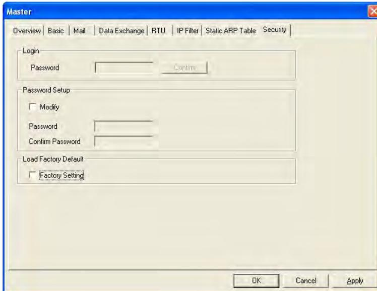
3. Select the **Modify** checkbox, and enter "aabb" in the **Password** box and the **Confirm Password** box. Click on **OK** to save the password.
