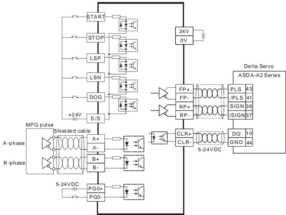
1. Please use 22-16AWG (1.5mm) wiring (either single or multiple core) for I/O wiring terminals. PLC terminal screws should be tightened to 1.90kg-cm (1.65lb-in). Use copper conductors only, 60/75oC.
