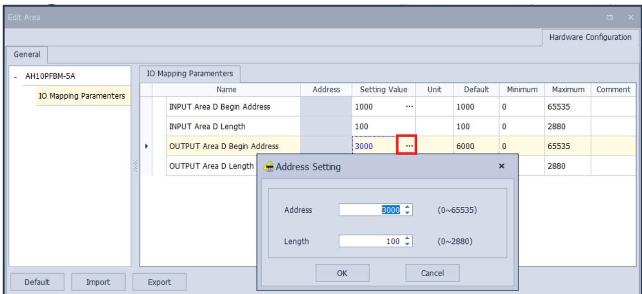
The diagram below illustrates the mapping addresses allocated by the master station for the slave configuration module parameters. By the upper and lower diagrams, it can be observed that the slave configuration module corresponds to the starting register numbers of the master PLC's OUTPUT and INPUT areas.
