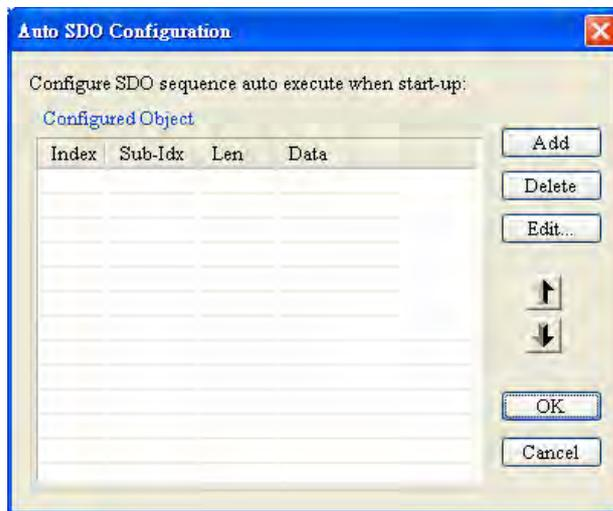
The following window pops up by clicking on "Add" button in the window above. "Index (hex)" and "Sub-Index (hex)" are the index and sub-index of the parameters to be accessed; "Length (dec)" is determined by the data type of the parameter to be accessed with the unit: byte.
