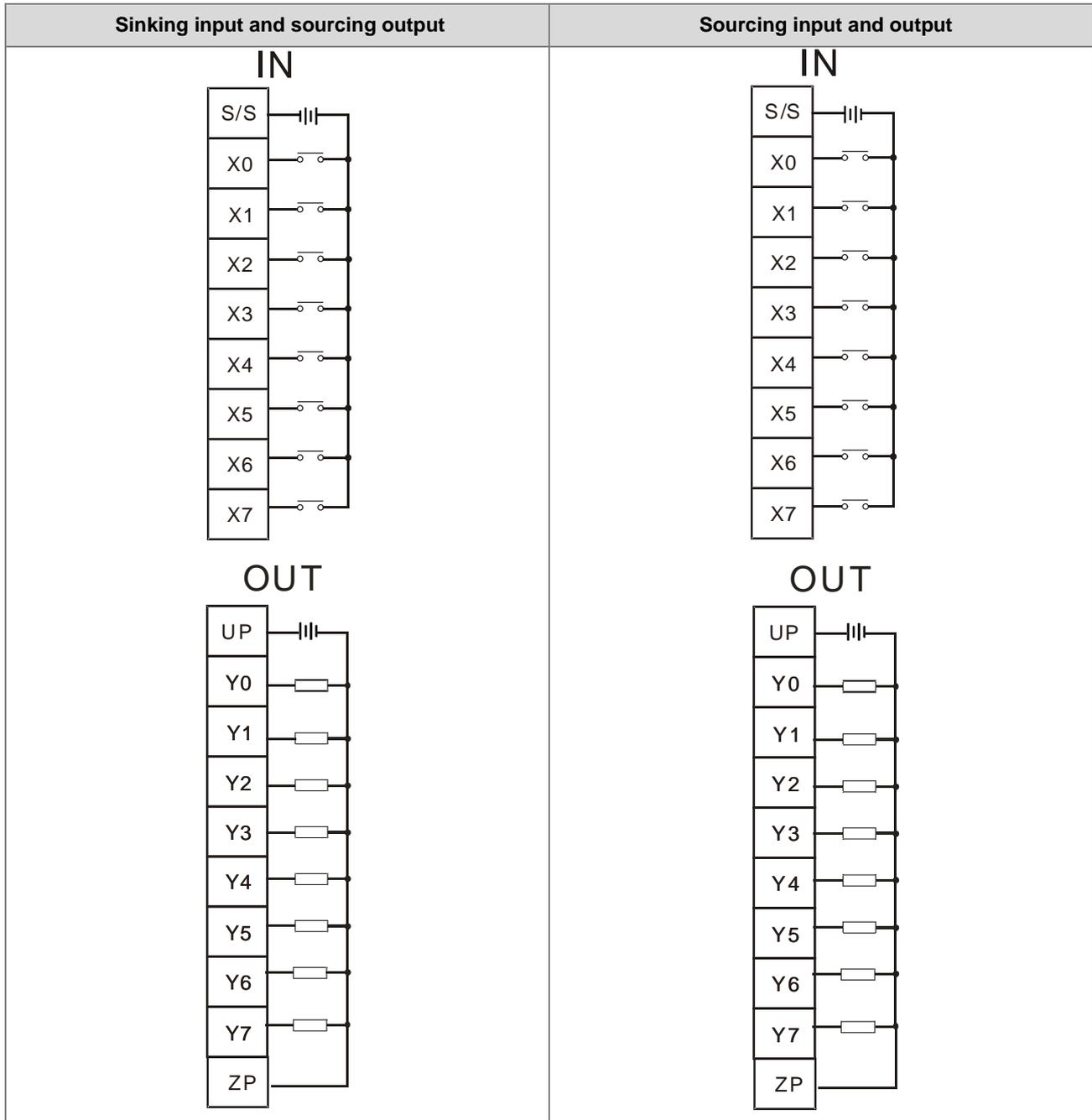
Note: You need to add external power supply 24 VDC (-15% ~ +20%) for UP and ZP; power consumption is up to 15 mA.
