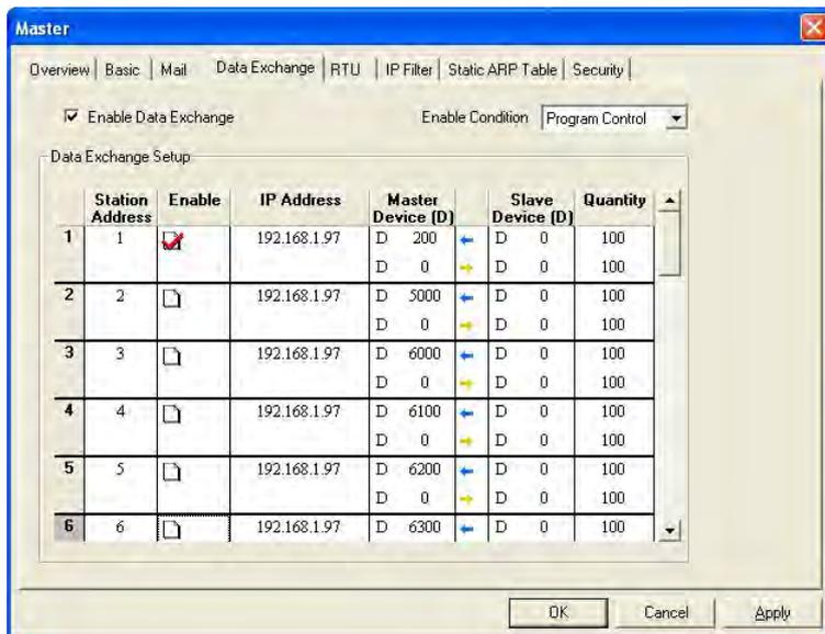
3. Select the **Enable Data Exchange** checkbox. Select Program Control in the **Enable Condition** drop-down list box. Enter the IP address of PLC\_A “192.168.0.4” in the **IP Address** cell corresponding to station address 1. Click on **Apply** to complete the setting.
