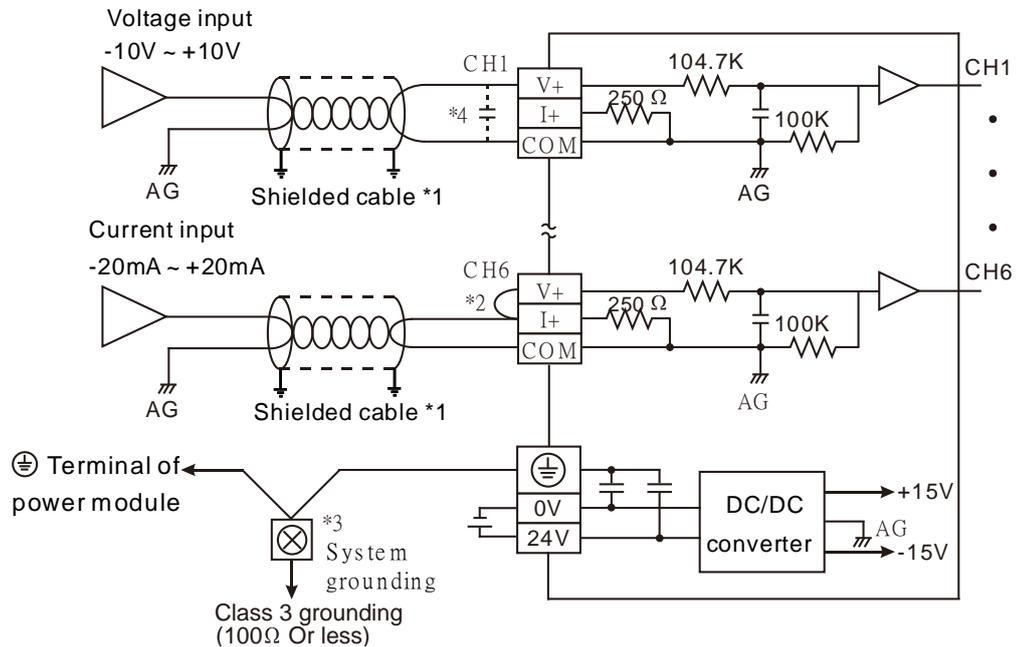
\*1: When performing analog input, please isolate other power wirings.
