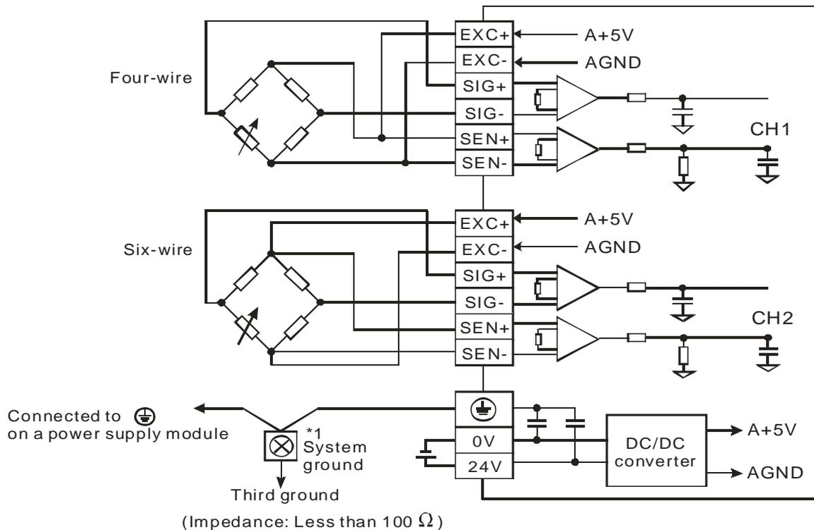
Note 1: Please connect  $\oplus$  on a power supply module and  $\oplus$  on the load cell module to a system ground, and then ground the system ground or connect the system ground to a distribution box.
