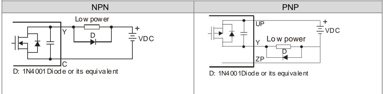
④ 2. A diode and Zener are connected in parallel to absorb the surge voltage: used in high-power and power-on/off frequently situations.
