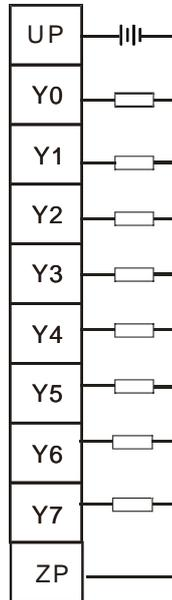
Note: You need to add external power supply 24 VDC (-15% ~ +20%) for UP and ZP; power consumption is up to 15 mA.
