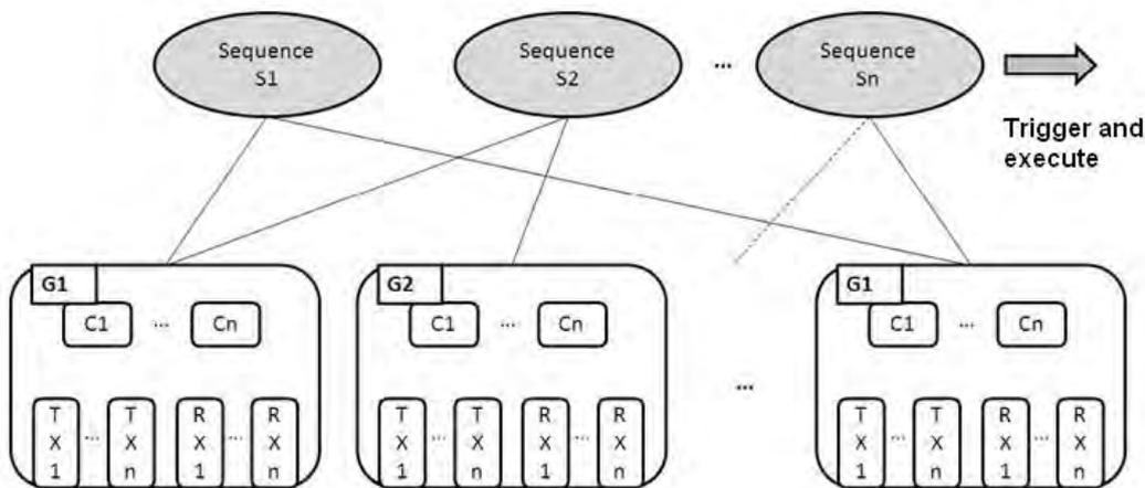
First of all, establish the transmission instructions (TXs) and the reception instructions (RXs) in the group. Then, set the execution sequence and the number of times for TXs and RXs through the commands. Finally, trigger and execute the instructions as a group. In addition, if various groups of group packets are required in a large system, the user can create the groups in the sequences, and set the execution sequence.
