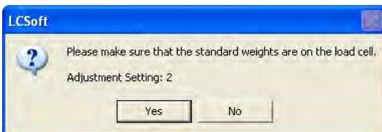
Step 6: Put a standard weight which weighs 1500 g on the load cell used. Type “1500” in the **Wight value of weights** box, type “1500” in the **Digital value of weights** box, and click **Next**. Please see the figures below.
