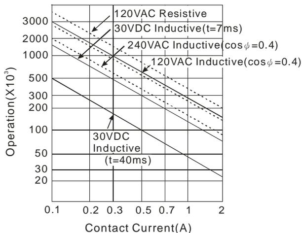
\*4. Life cycle curve: The lifetime of a relay terminal varies with the working voltage, the load type (the power factor  $\cos\phi$ ), the time constant  $t(L/R)$ , and the current passing through the terminal. The life cycle curve is shown below.
