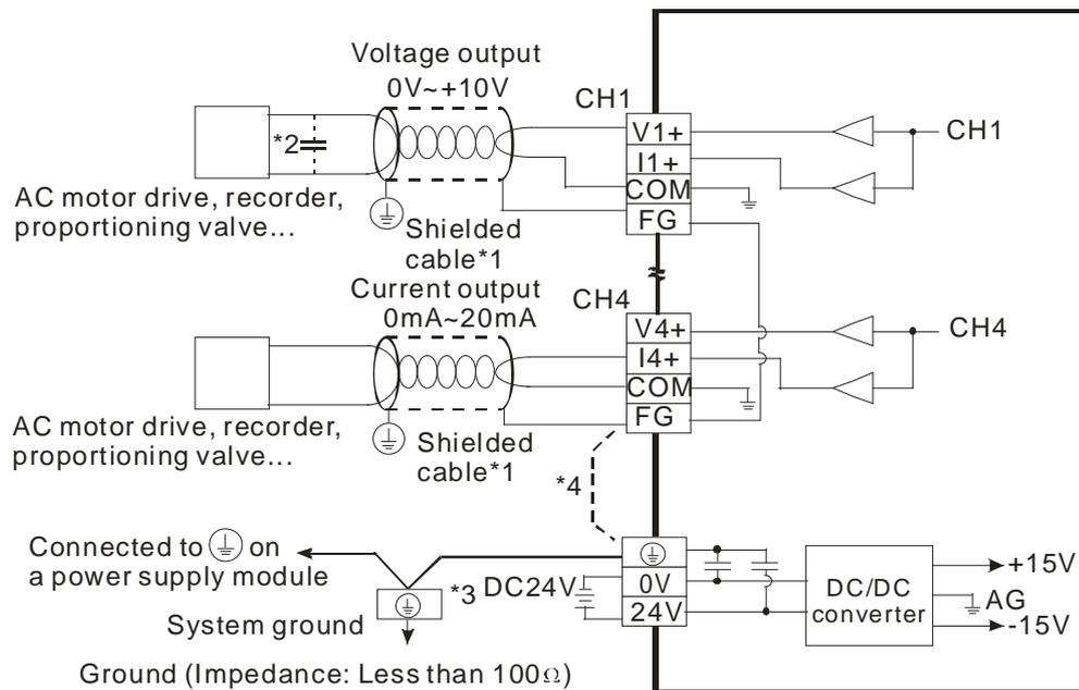
Note 1: Please isolate the analog output cable from other power cables.
