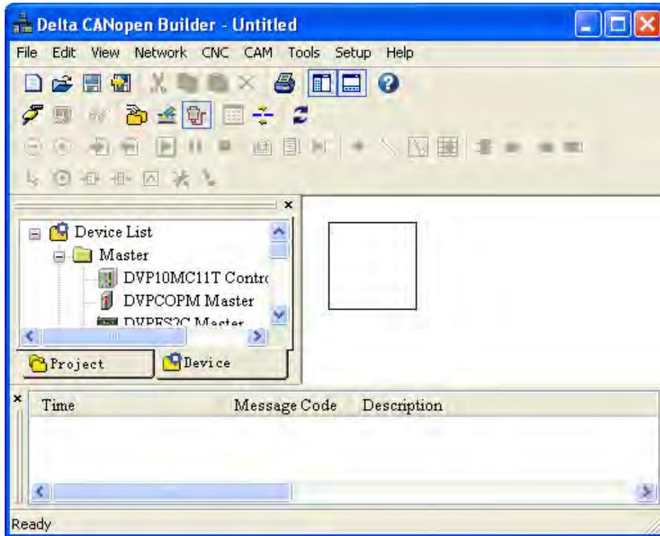
2. Select "Setup" => "Communication Setting" => "System Channel", and the "Serial Port Setting" dialog box will appear.
