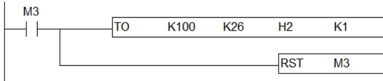
Step 8: Make sure that the value displayed is correct, and make the adjustment retentive. Write H'5678 to CR#41. Please see the WPLSoft program shown below.
