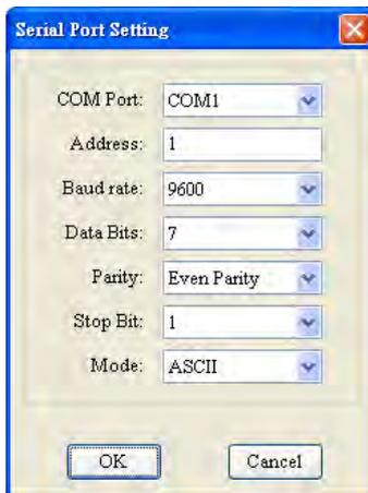
2. Set up the communication parameters for the PC and DVP-SV, e.g. the communication port, address, baud rate and communication format. Click on “OK” after the configuration is finished.
