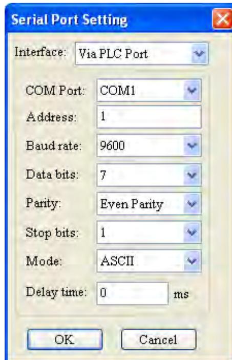
3. Set up the parameters for communication between the PC and DVP-SV, e.g. the communication port, address, baud rate and communication format.
