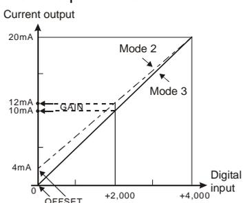
Mode 2 of CR#1:  $\text{GAIN}=12\text{mA} ( 2,400_{\text{LSB}} ) \cdot \text{OFFSET}=4\text{mA} ( 800_{\text{LSB}} ) .$
