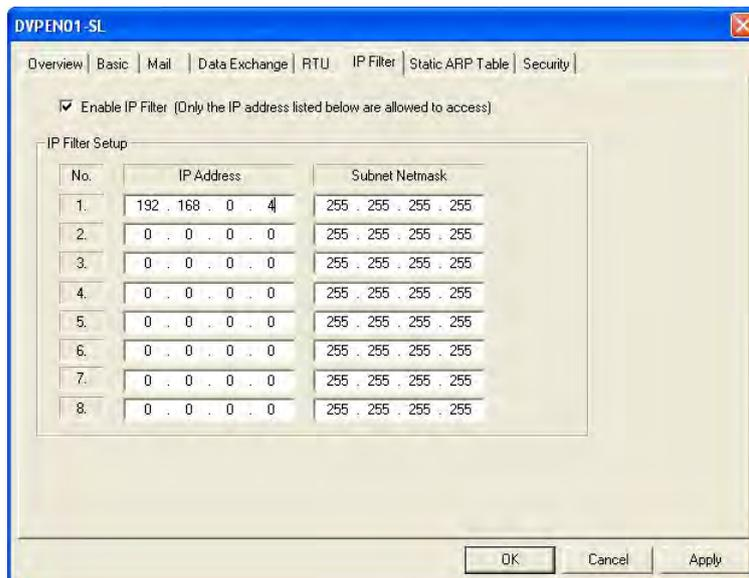
3. Select the **Enable IP Filter** checkbox. Enter “192.168.0.4” in the **No. 1 IP Address** box and “255.255.255.255” in the **No. 1 Subnet Netmask** box.
