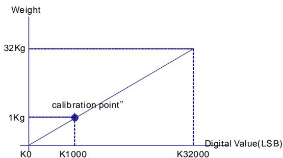
The digital values corresponding to the calibration weight can be written arbitrarily by the user, and the generated curve graph will also differ. For example, if you modify the 1kg calibration weight corresponding to K1000 to 1kg corresponding to K500, write it into CR#33 (CH1 calibration weight baseline), as shown in the WPLSoft program in the following diagram.
