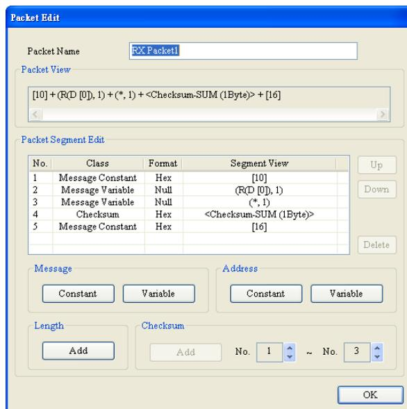
Edit the SCM command: Sending Tx Packet1 and receiving Rx Packet1.
