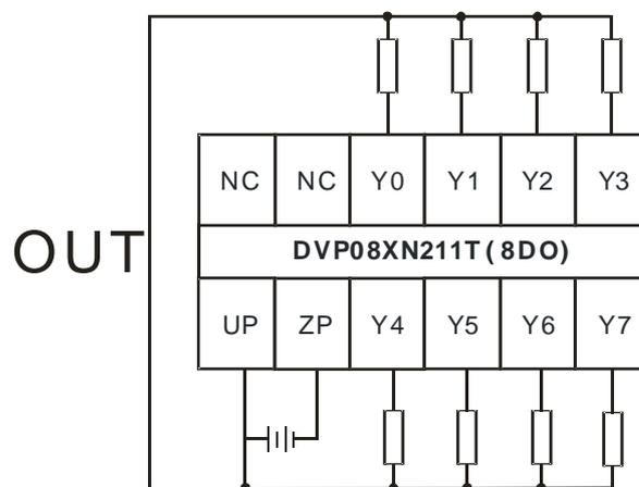
Note: You need to add external power supply 24 VDC (-15% ~ +20%) for UP and ZP; power consumption is up to 10 mA
