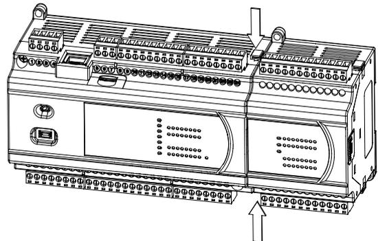
1.3.2.2 Connection and Installation of DVP-S Series PLC and Modules
