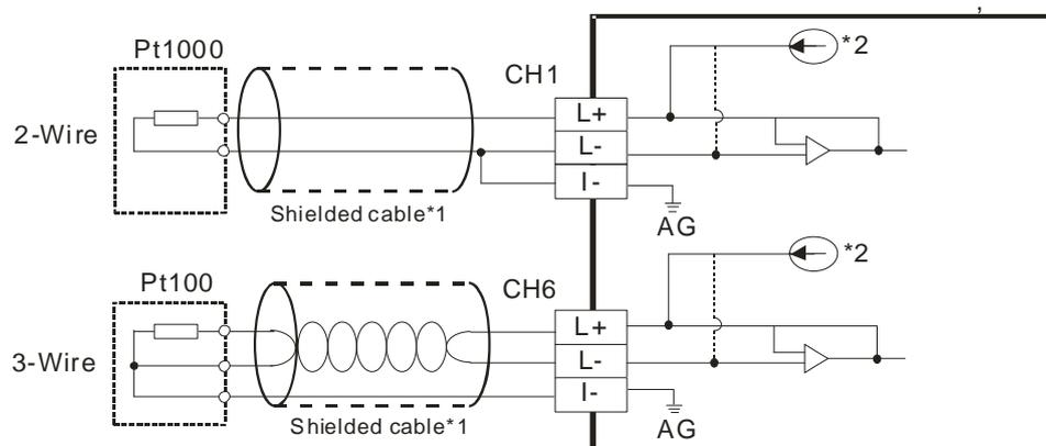
Note1: Use only the wires that are packed with the temperature sensor for analog input and separate from other power line or any wire that may cause noise.
