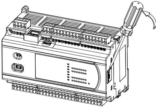
Step Two: Use a flathead screwdriver to pry open the locking tab of the I/O module.
