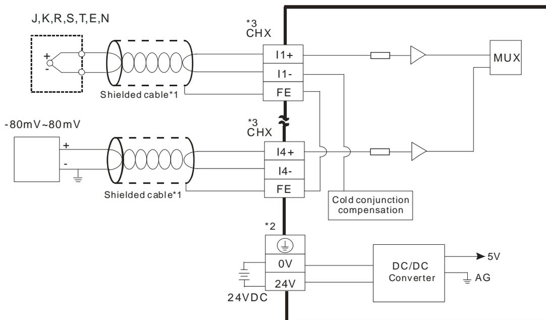
\*1. The cable connected to the input terminal should be the cable or the shielded twisted pair cable connected to a type J, K, R, S, T, E, N thermocouple. It should be kept separate from other power cables and cables that generate noise.
