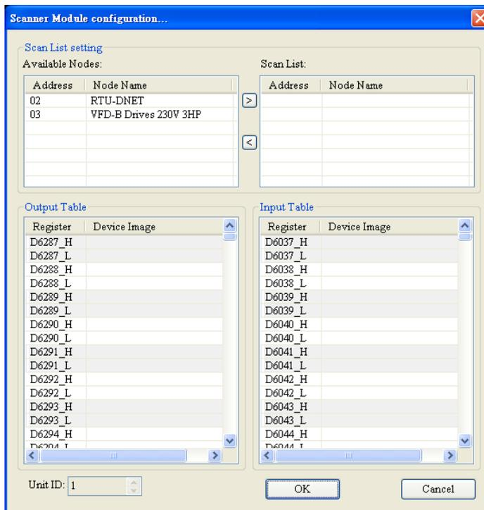
2. Move the DeviceNet slave devices in the "Available Nodes" list on the left side to the "Scan List" on the right side. Select one node and click on [>]. In this way, move all the nodes to the scan list.
