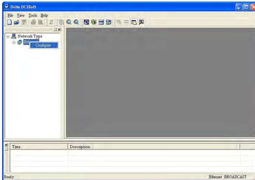
2. After configuring a model, select the DVPEN01-SL checkbox and click OK to auto-search for DVPEN01-SL modules on the network.
