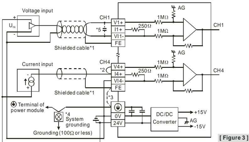
Note 1: When performing analog input, please isolate other power wirings.
