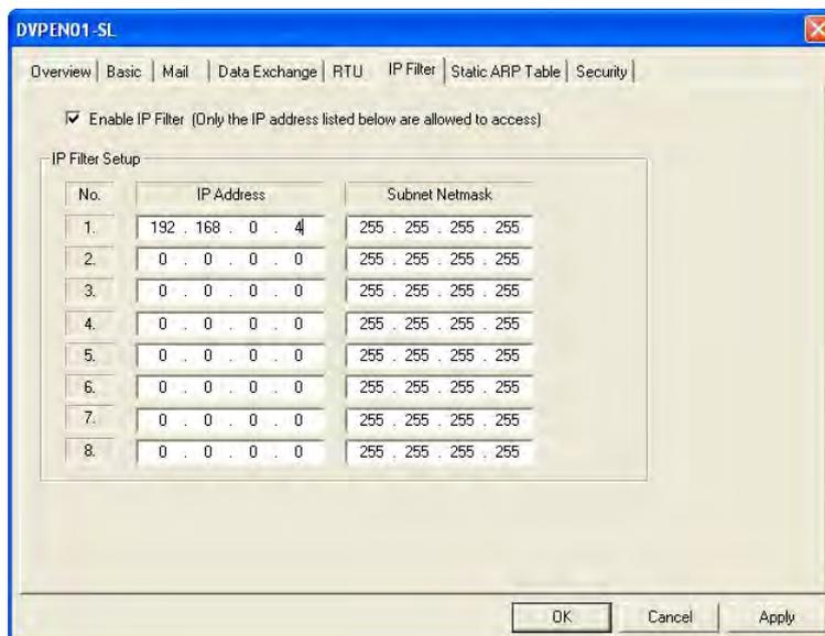
4. Enter "192.168.0.1" in the **No. 2 IP Address** box and "255.255.255.0" in the No.2 **Subnet Netmask** box. Click on **OK** to complete the setting. Only the equipment within the IP address range can be connected.
