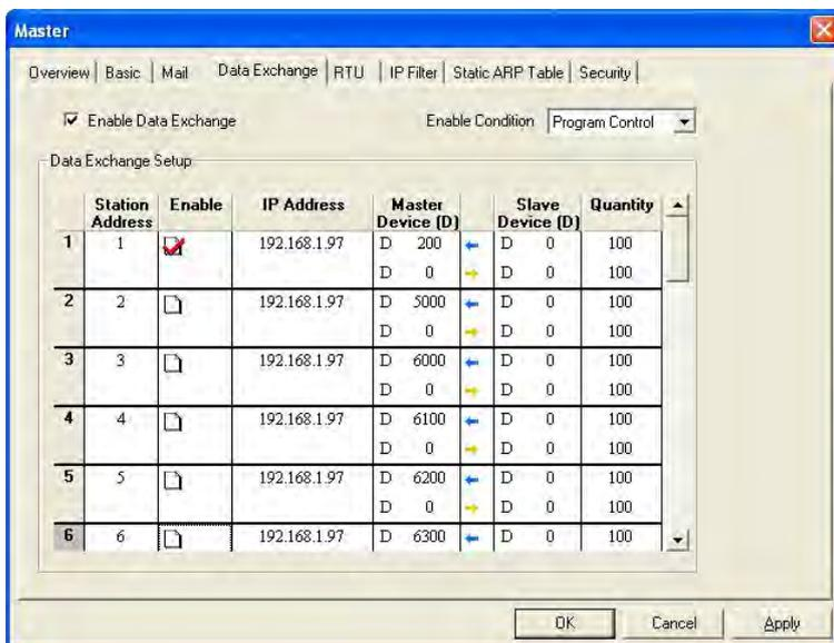
3. Check '**Enable Data Exchange**,' select the execution mode as '**Program Control**.' Check the '**Enable**' option for the first data exchange group, enter PLC\_B IP as '192.168.1.97' in the first IP address of the group. Set D200←D0 and D0→D0, both with a quantity of 100 records.
