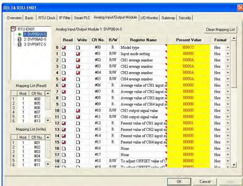
3. Use DCISoft for DVPEN01-SL to set start addresses and numbers. (RX: M2000~M2009; RY: M3000~M3009; RCR (Reading): D2000~D2009; RCR (Writing): D3000~D3009)
