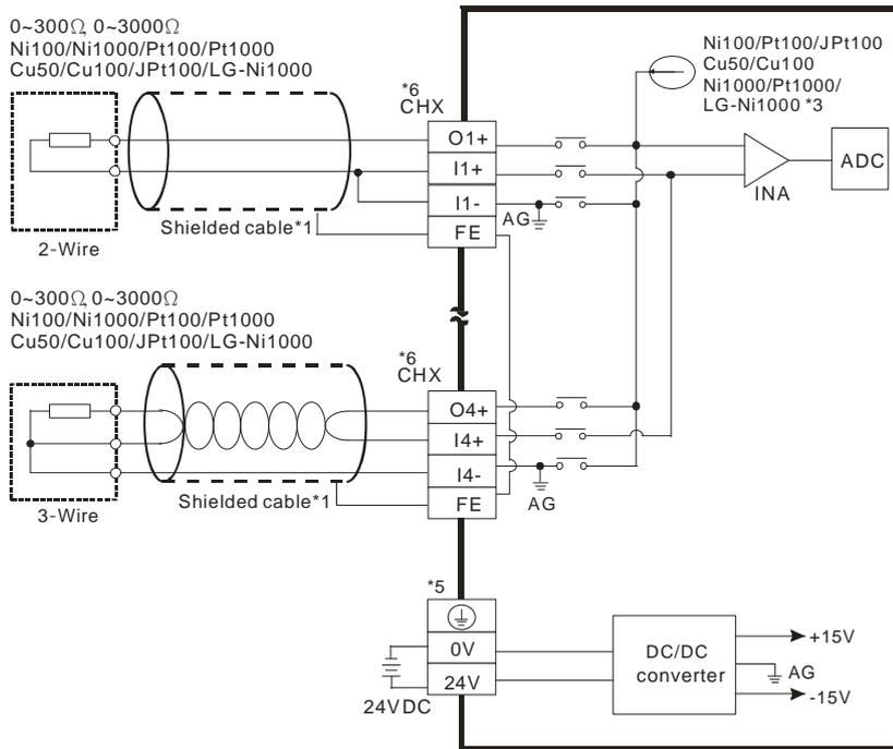
\*1. Use shielded twisted pair cables for temperature sensors, including Ni100/Ni1000, Pt100/Pt1000, Cu50/Cu100, JPt100, LG-Ni1000 for analog input module wiring and keep them away from power cables and other cables that generate noise. Use 3-wire temperature sensors. But if you use two-wire temperature sensors, In+ and In- must be short-circuited (where n is between 1–6).
