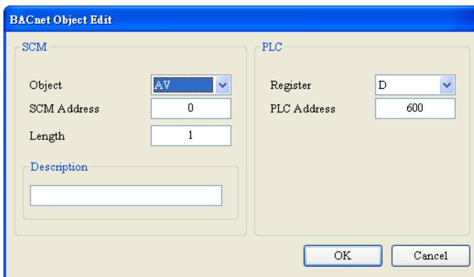
Object: You can select "AV" or "BV". "AV" corresponds to the data registers in the PLC, and "BV" corresponds to the coil in the PLC.
