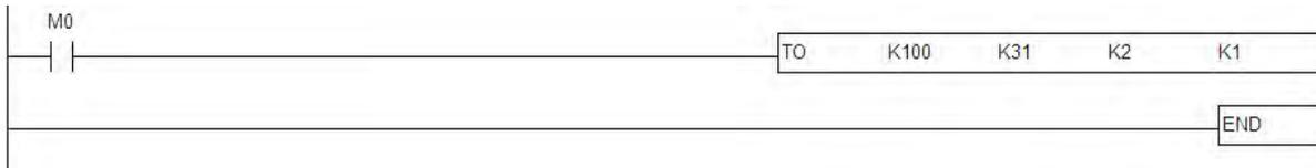
After M0 is triggered, COM1 on the SCM module will keep reading the present value which will be stored in D100, and the status value of bit0 in D0 is 1.
