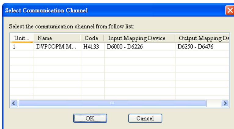
If there are more than one DVPCOPM-SL module (less than 8) connected to the left side of DVP-SV and suppose there are two connected in this example, you will see the screen as below after clicking on "Online". The DVPCOPM-SL which is closest to DVP-SV is regarded as the first module, and so on.
