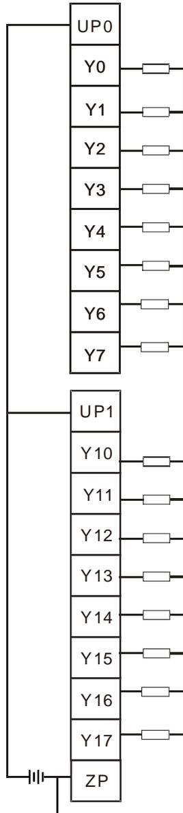
Note: You need to add external power supply 24 VDC (-15% ~ +20%) for UP0, UP1 and ZP; power consumption is up to 25 mA.
