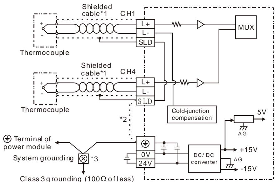
Note1: Use only the wires that are supplied with J, K, R, S, T thermocouple sensor. Tighten PLC terminal screws to a torque of 1.95 kg-cm (1.7 in-lbs).
