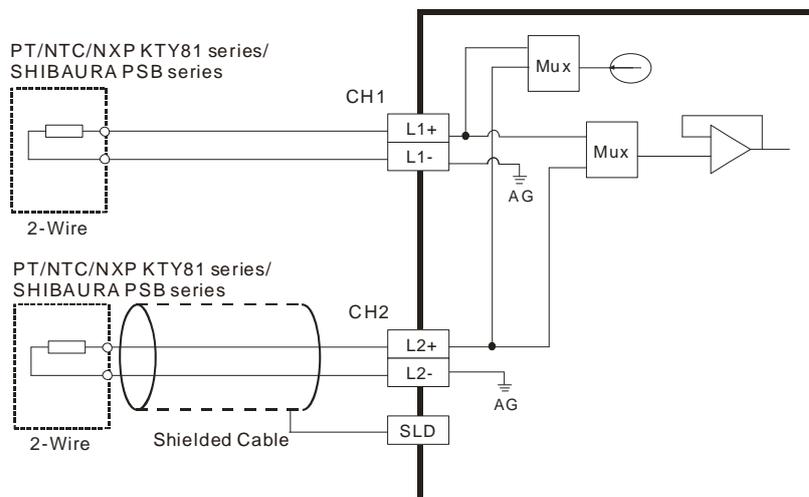
Note1: Use only the wires that are packed with the temperature sensor for analog input and separate from other power line or any wire that may cause noise.
