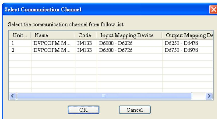
Select the DVPCOPM-SL which needs to establish the communication. Click on “OK” and start to scan all the slaves in the network. If the network installation and power supply are normal, you will see the screen as below.
