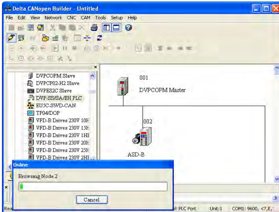
5. In normal condition, after the scan is over, you will find the master and all the slaves displayed in CANopen network, as below.
