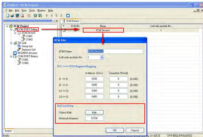
BACnet object edit: Editing the AV and BV values which correspond to the data registers and coils in the Delta PLC master connecting to the SCM module
