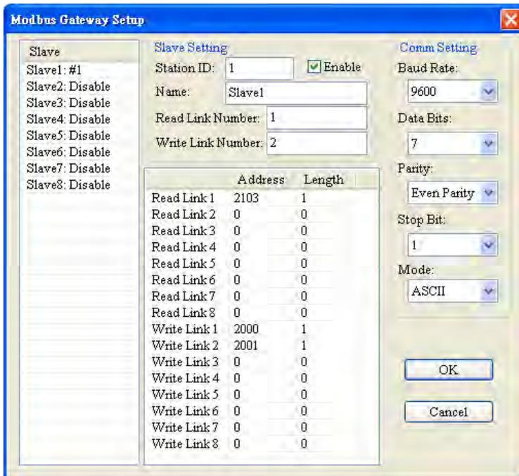
Note: The slave mentioned here is the slave on the Modbus network and has nothing directly to do with the DeviceNet network.
