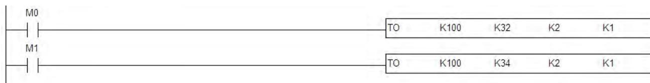
After M0 is triggered, the data will be read from the slave address which has been set through COM2 on the SCM module.
