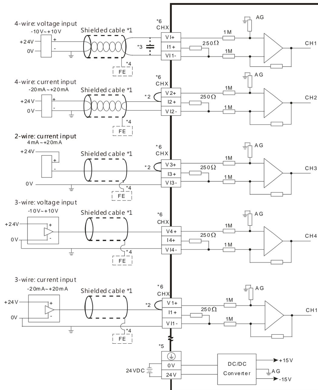
\*1. Use shielded cables to isolate the analog input signal cable from other power cables
