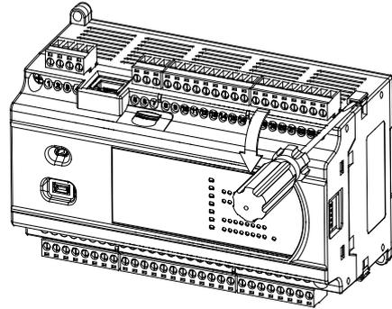
Step Three: Connect the PLC I/O module connector port with the module connector port.
