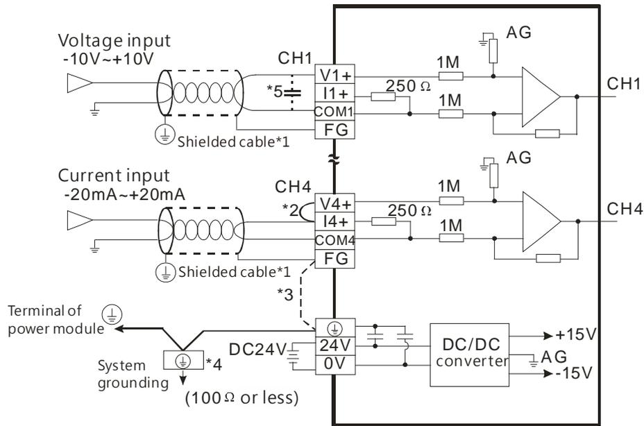
\*1: When performing analog input, please isolate other power wirings.
