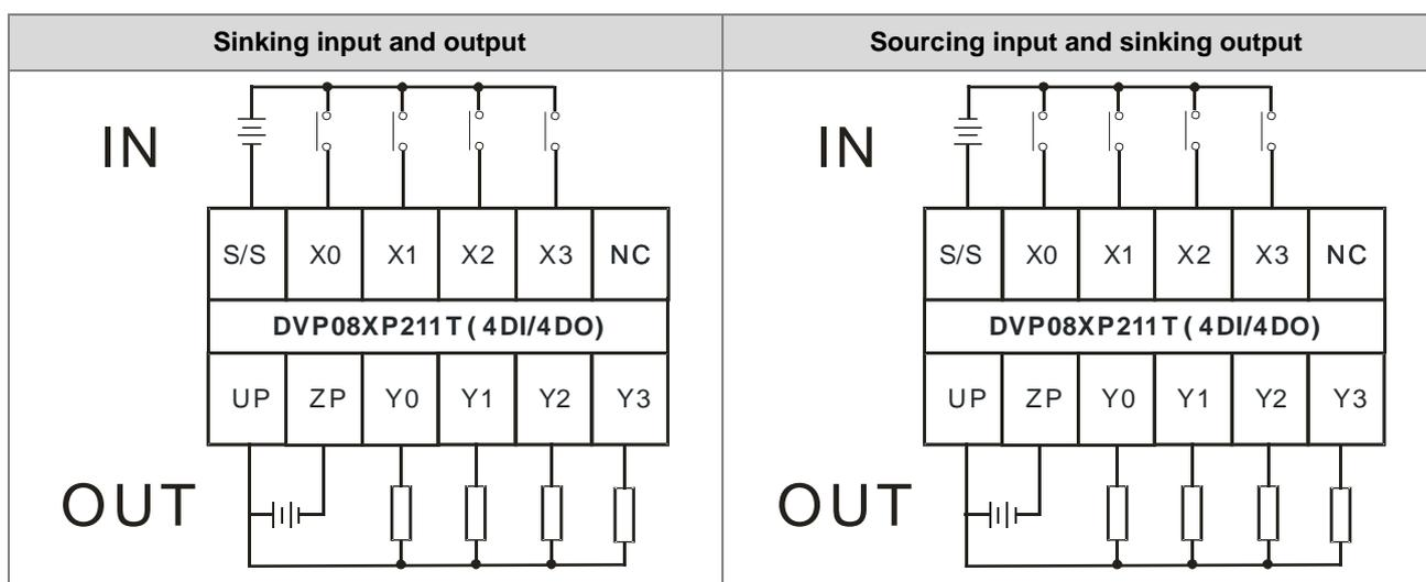
Note: You need to add external power supply 24 VDC (-15% ~ +20%) for UP and ZP; power consumption is up to 5 mA.
