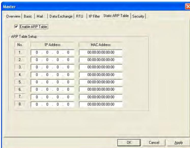
3. Select the **Enable ARP Table** checkbox. Enter "192.168.1.6" in the **No. 1 IP Address** box, and its corresponding MAC address is "00:18:23:10:00:35".
