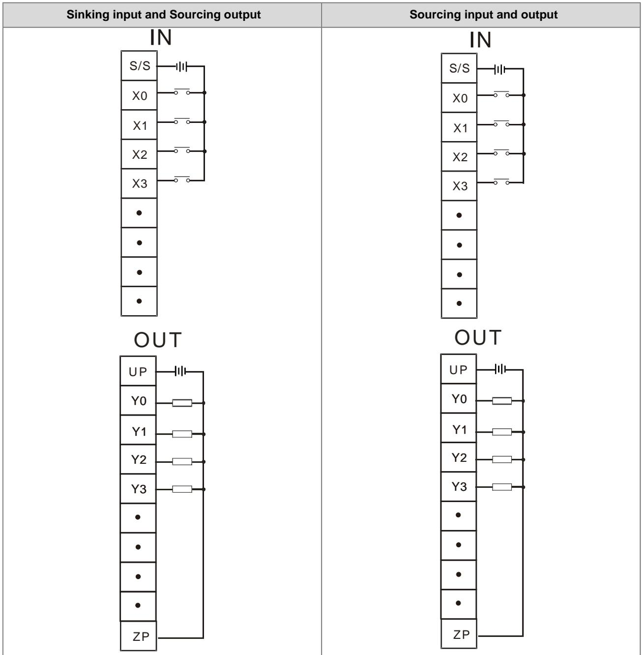
Note: You need to add external power supply 24 VDC (-15% ~ +20%) for UP and ZP; power consumption is up to 10 mA.
