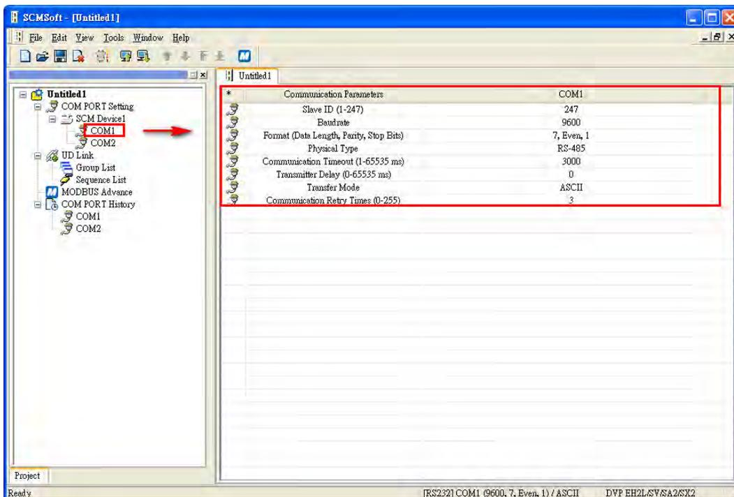
Set the communication parameters of COM1: station address 247 (default), Modbus RTU, 9600, 8, Even, 1.
