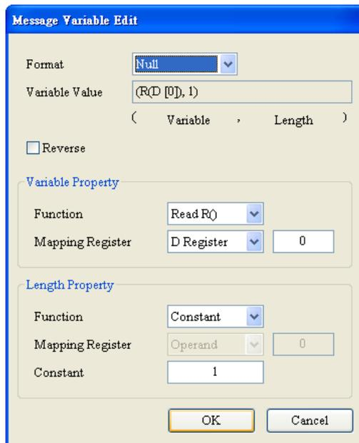
Note: Some unimportant words can be ignored. You can just store the data which is needed in the registers (Dx), and the data whose length of the response code is unknown can be stored in the registers by means of this method.
