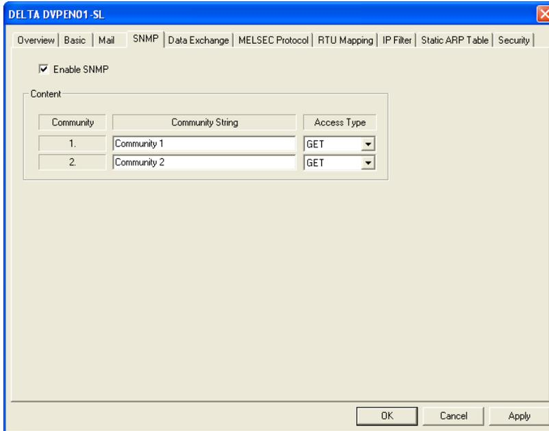
1. **Enable SNMP:** Disable/enable the SNMP function.
