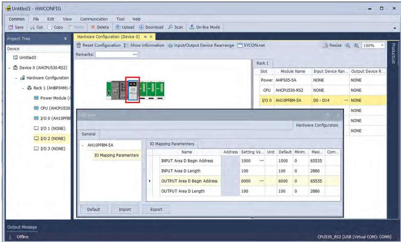
The diagram below illustrates the starting addresses and lengths of the OUTPUT and INPUT areas assigned by the master module for the master PLC. Data from the OUTPUT area is transmitted to the slave, while the INPUT area receives data sent from the slave.
