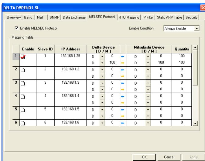
※ After the settings are downloaded, DVPEN01-SL will read the data in D0~D99 in the Mitsubishi PLC into D0~D99 in DVP28SV, and write the data in D100~D199 in DVP28SV into D100~D199 in the Mitsubishi PLC.
