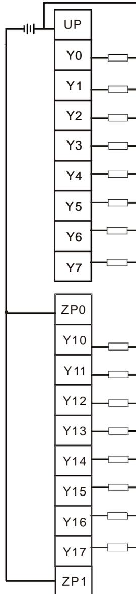
Note: You need to add external power supply 24 VDC (-15% ~ +20%) for UP, ZP0, ZP1; power consumption is up to 30 mA.
