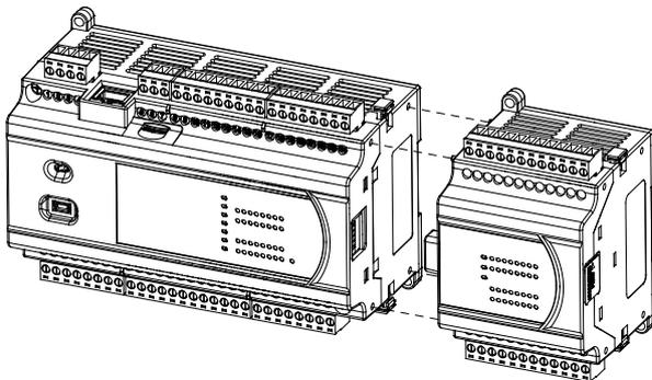
Step Four: Press the upper and lower locking tabs of the I/O module in the direction of the arrow to secure the modules in place.
