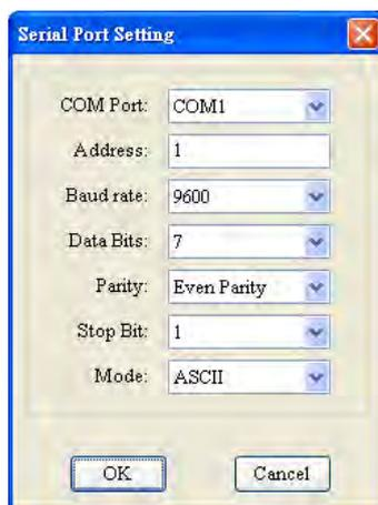
3. Set up the communication parameters for the PC and DVP-SV, e.g. the communication port, address, baud rate and communication format. Click on "OK" after the configuration is finished.
