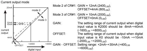
The charts above are D/A conversion characteristic curve of voltage input mode and current input mode. Users can adjust conversion characteristic curve by changing OFFSET values (CR#18~CR#21) and GAIN values (CR#24~CR#27) depend on application
